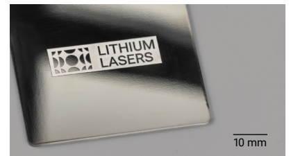
100 µm deep stainless steel engraving with white finish
