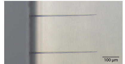
High-aspect-ratio drilling in fused silica
